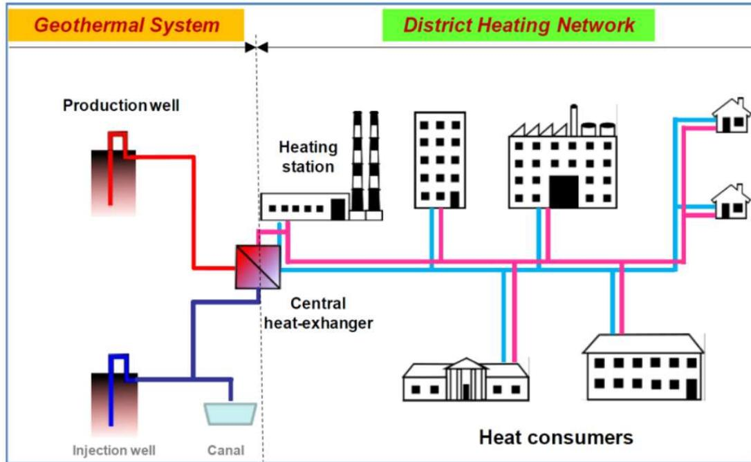
Scheme of geothermal based district heating
