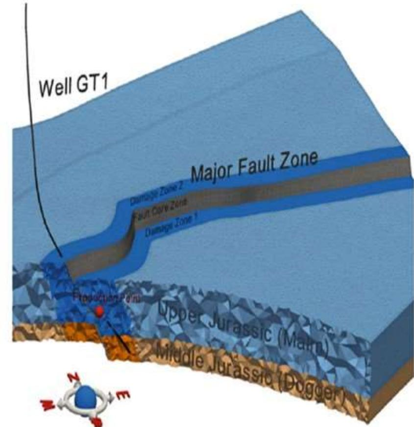
(a) Geometry of the model considering a production well within the damage zone
