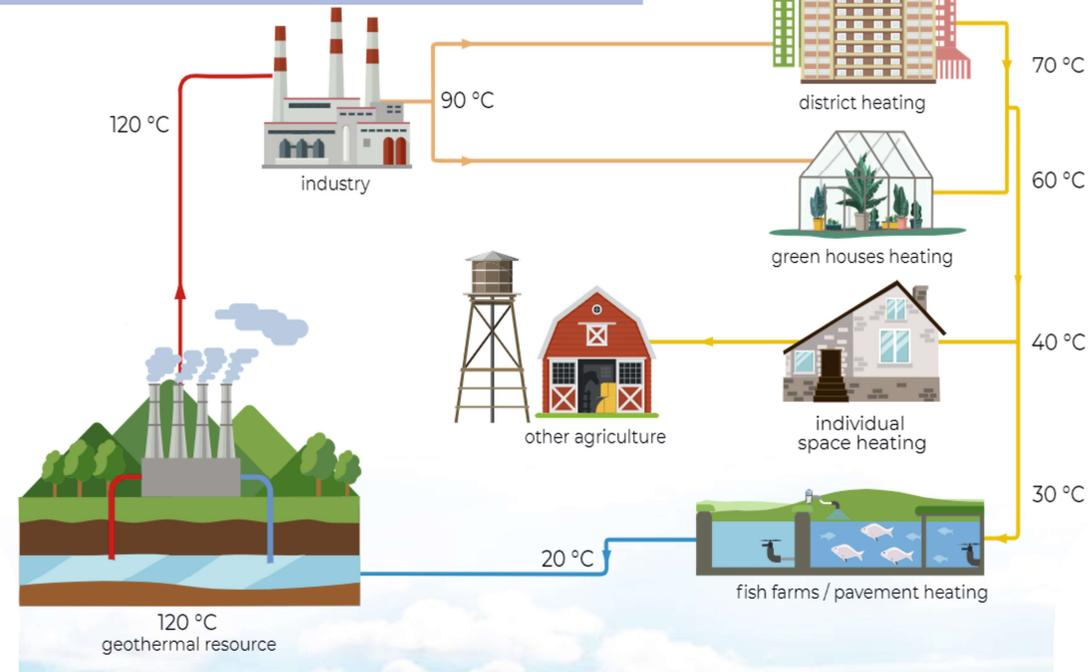
Sketch of an ideal geothermal cascade system where users are sequentially linked according to their decreasing heat demand
